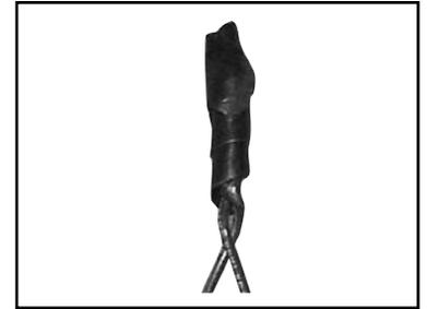
Using just electrical tape is not sufficient. The wires may become corroded or vibrate loose creating a short.
