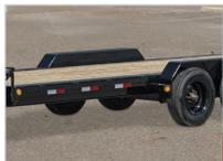
Our Torsion Drop Axles effectively minimize deck height while utilizing a 10" frame beam, creating a more accessible loading surface for vehicles and equipment without compromising structural integrity.
