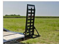
Choose from various ramp options, including Fold-Up Ramps (Shown) and optional Monster Ramps with Hold-down Latches, to enjoy enhanced strength and loading flexibility for both equipment and vehicles.
