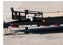
Experience unmatched strength with our 8" channel frame and tongue, designed for heavy-duty performance and durability, ensuring a reliable and robust foundation for transporting vehicles and equipment.
