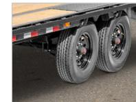
Our 8K Axles feature Forward Self-Adjusting Brakes for optimal stopping power. The Oil Bath Hubs and Valcrum Caps simplify axle maintenance, enable easy oil level checks, and eliminate concerns about broken plastic caps.
