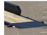
Our 30" Diamond plate knife edge tail makes it super-easy to load low clearance equipment like scissor lifts and fork lifts.
