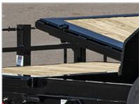
Our Gravity Tilt uses a hydraulic cylinder and proportioning valve to control the rate of tilt movement for additional safety when loading and unloading.
